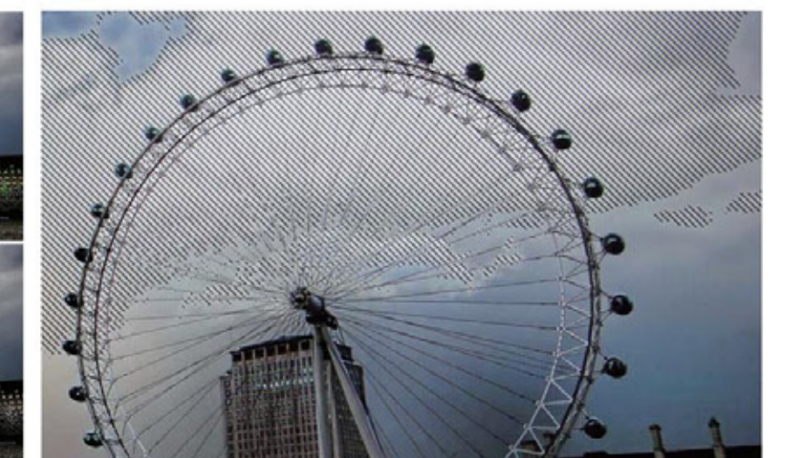
Areas of image over a certain threshold are filled with striped pattern to dramatically highlight areas where too much light is falling on image sensor.
