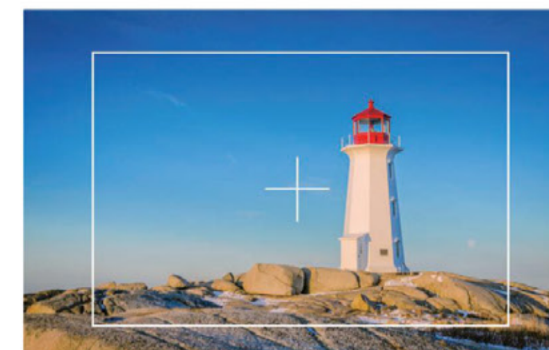
Adjusts a wide range of aspect marker, safety marker and center marker. It can also weaken the sense of the image outside the marker.
