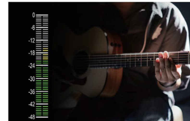
The figure on left side of screen displays level meter showing audio levels for channels 1 and 2 of the input source.
